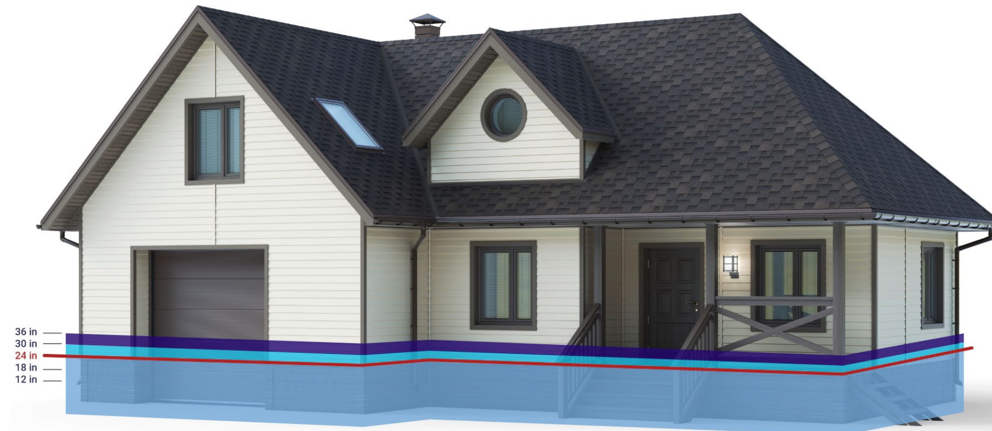
24 inches first floor elevation. No damage inside the home below 24 inches.
